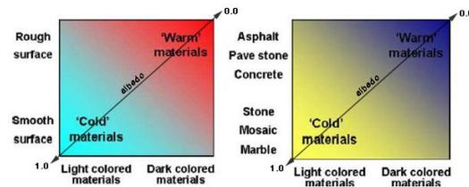
**Fig. 2:** Definition ‘cool’ and ‘warm’ material based on physical characteristics (color, surface texture and material) and albedo value [14].
